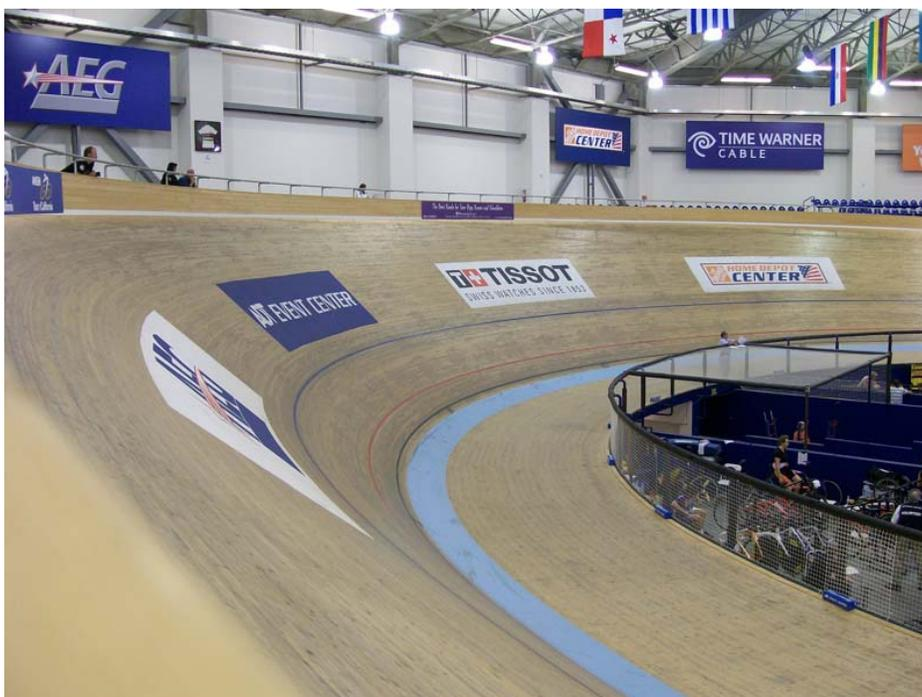
Tracks vary in length, banking and other characteristics. The picture above is of the 250-meter indoor track at the ADT Center in Carson, California where many elite races are held in the United States. Looking at the picture, you can see pretty clearly how steep the banking is – just shy of 45°. The straightaways are also banked, but not nearly as much. Shorter tracks can be even steeper than this one, and longer tracks are invariably less steep in the corners.
